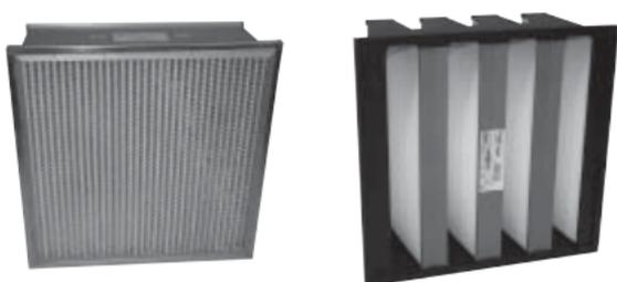
Both filters are 24" by 24" by 12", the filter on the right has double the media area of the filter on the left. The filter on the right will last longer and offer significant energy savings. At 10¢ a kilowatt hour the filter on the left will cost \$127.90 per year to operate and the filter on the right will cost \$53.50 (2000 cfm per filter & 60% fan efficiency). Some bag filters can cost up to \$238.60 per year in energy.
