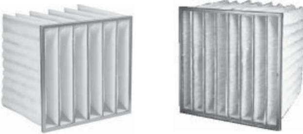
The filter on the left has 6 pockets, the filter on the right has 8 pockets, and both are the same length. The filter on the right has 30% more media area and will last longer and use less energy in its life within the system. At 10¢ a kilowatt hour the filter on the left will cost \$95.00 per year to operate and the filter on the right will cost \$56.00 (2000 cfm per filter & 60% fan efficiency). Some bag filters can cost up to \$227.00 per year in energy.
